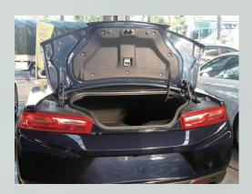
4. Remove the clips securing the trim panel on top of the tail lights. Remove the board and set aside. 2. Remove the four (4) nuts holding the trunk trim on around the latch and remove the trim panel. Set aside.
