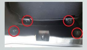
3. Remove the interior panel trim clips with a Y-shaped trim removal tool or carefully with a flathead screwdriver.
